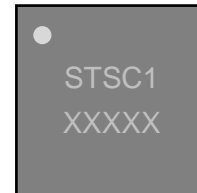
Figure 7 Laser marking on STSC1, the top line with the pin-1 indicator and the sensor type, the bottom line with the 5-digit alphanumeric tracking code.
