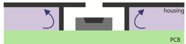
Figure 2. Separating a sensor compartment from the remaining housing minimizes the influence of entrapped air on the sensor.
