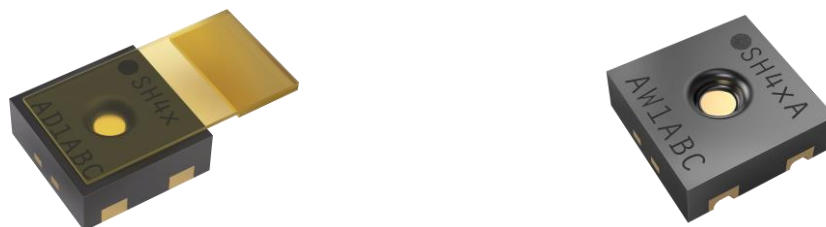
Figure 16. Left: SHT4x protective cover option. Right: SHT4xA (automotive grade) with wettable flanks.
